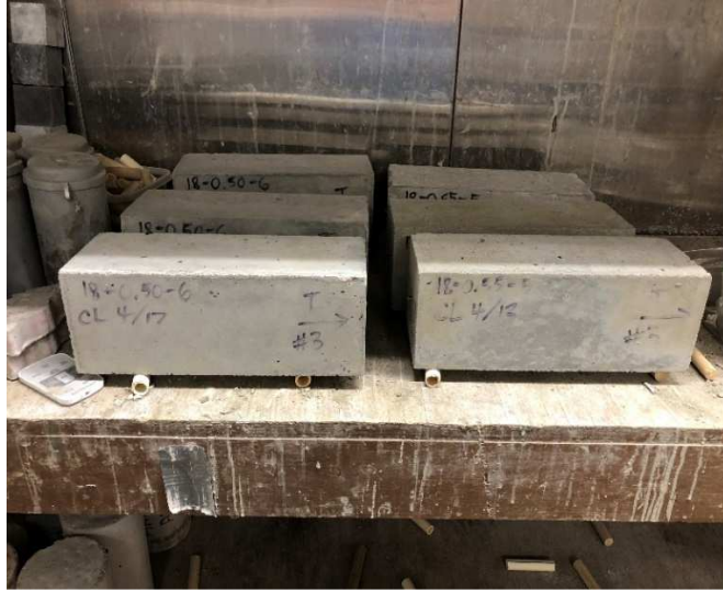
Figure 3.1. Drying Shrinkage specimen
