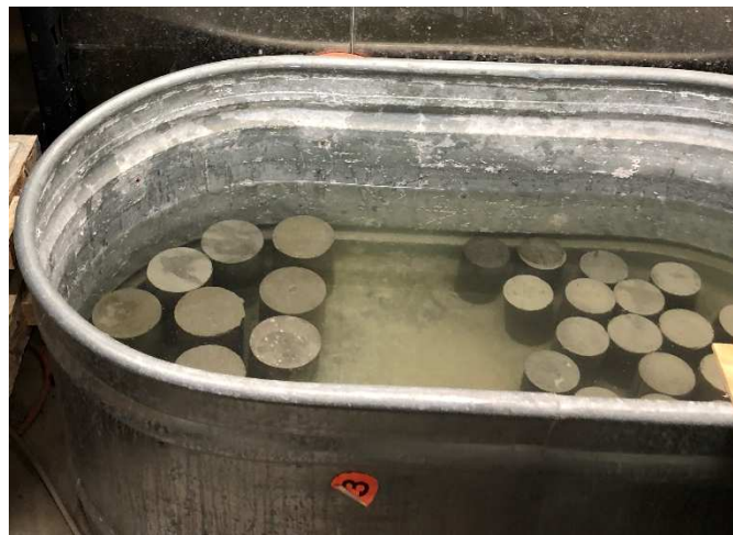
Figure 3.2. Compressive Strength specimen
