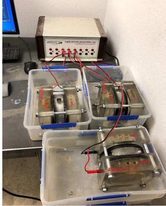
Figure 3.6. Rapid Chloride Ion Permeability testing
