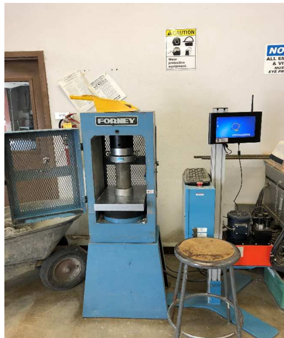
Figure 3.3. Compressive Strength Testing
